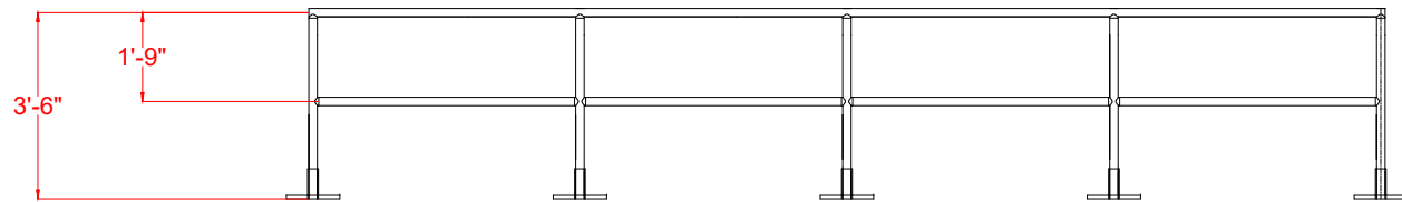
TYPICAL 20' SECTION ALUMINUM PIPE
