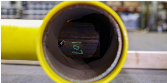
**5.** Back out the two bolts that are installed on the 4" horizontal rail 1 ½" [11 turns] and replace the two caps on the posts.
